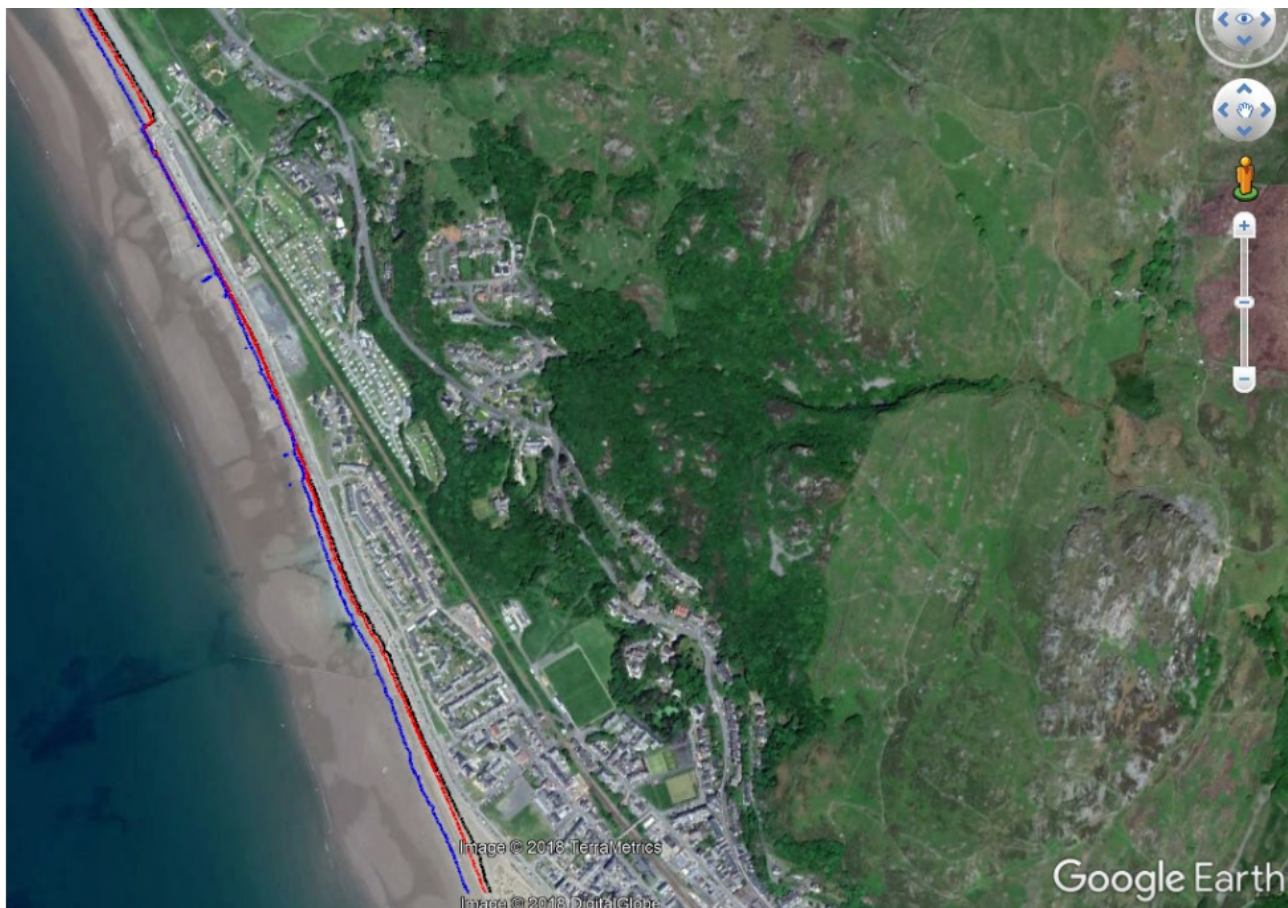
Graphic 12-1 Aerial Image of North Promenade showing coastline for different existing tidal levels (MHWN =1.3 mODN in blue, MHWS = 2.6 mODN in red, HAT 3.3 mODN in black), ODN Datum
