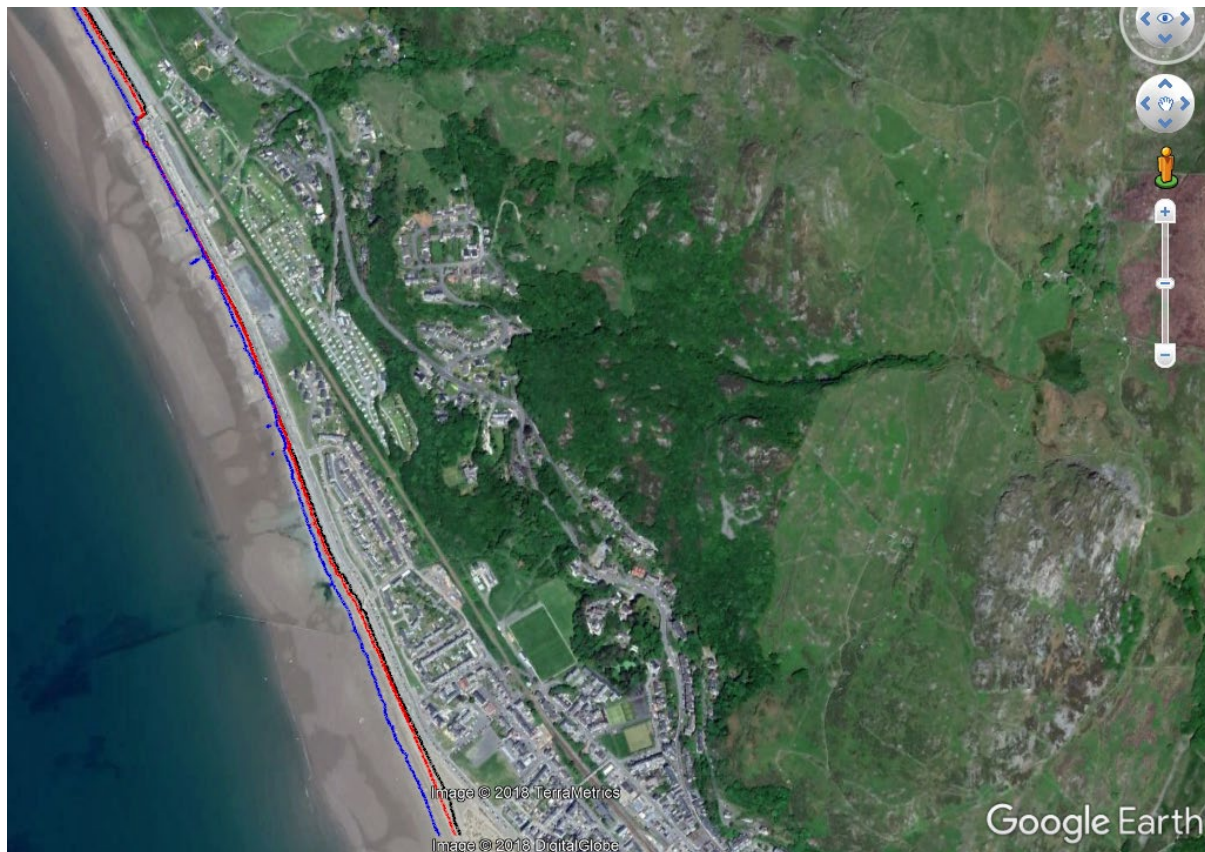
Figure 28. Aerial Image of North Promenade showing coastline for different existing tidal levels (MHWN = 1.3 mODN in blue, MHWS = 2.6 mODN in red, HAT 3.3 mODN in black), based on the composite DSM
